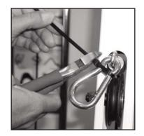
Slide end through hole, tighten. Cut off end of zip tie.
